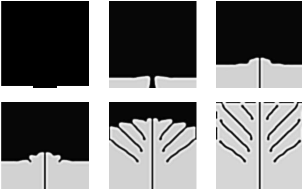
Figure 8.10: The evolution of two fronts in 2D, induced at the lower boundary of the grid. The upper left figure shows the initial state and the successive figures on the right and in the lower row illustrate the emerging morphological instabilities and the remaining stable domains of the initial state (black) at different times.
